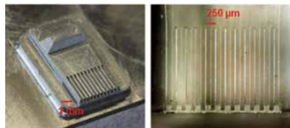
Fig.1: Metal master for the multi-channel system (left) and optical coupler (right)
