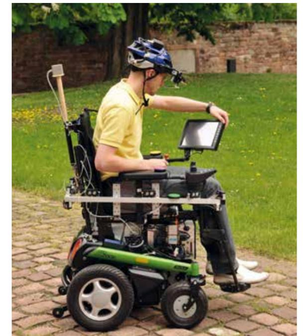
Fig.2: Assistance Wheelchair System based on a conventional electrical-powered wheelchair B600 (OttoBock Healthcare GmbH). The wheel-chair is equipped with a number of additional sensors and a real-time control computer.
