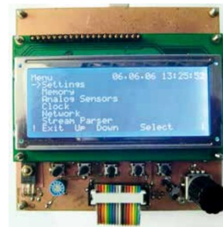
Fig.4: LCD display
