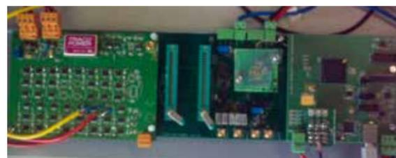
Fig. 2: Setup for measurements with the DSSC pixel ASIC with DEPFETs: A small piggy back board with the ASIC (center, light green) is connected to a base board which has two ZIF connectors to hold a
