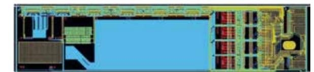
Fig.4: Layout of the electrical dummy module ( $\sim 1.5 \times 15 \text{ cm}$ ). The sensor matrix will be at the bottom right, 6 Switcher chips are located at the top, and 4 DCD readout chips and 4 data handling processor ASICs on the right. A flexible capton cable will be glued and bonded at the right end.
