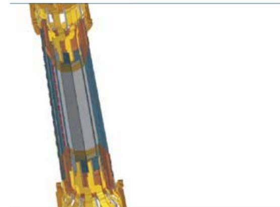
Fig. 2: PXD Design. The (gray) active module layers will be placed around the beam pipe (not shown) at radii of 13/22mm.
