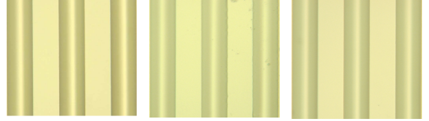
Fig. 1: Cylindrical micro lenses, left: in resist, middle: in PDMS, right: in UV-hardenable acrylate.
