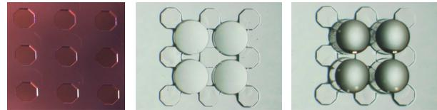
**Fig. 3:** Left: SU-8 mounting structure; Middle: GRIN-lenses on the image side; Right: GRIN-lenses on the object side
