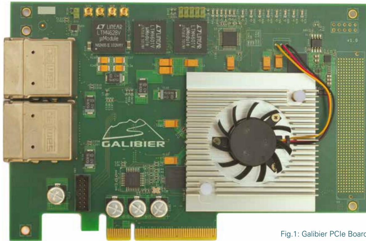
Fig.1: Galibier PCIe Board
