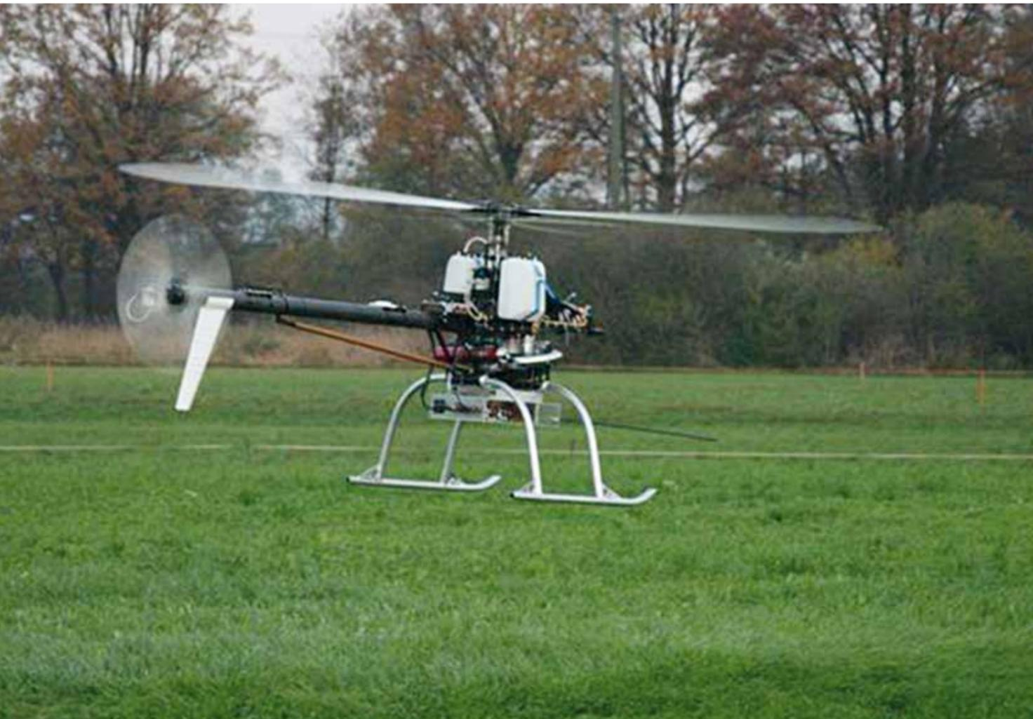
Fig.1: Autonomous Helicopter from Aeroscout type Scout B1-100.
