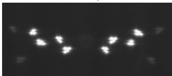
c) medium too far away from the front lens Fig. 2 Diffraction pattern of diffractive element
