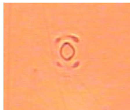
Fig. 5: pattern after double exposure. The spot diameters are 5 \mu\text{m} . The shift of the spots is less than 2 micron.
